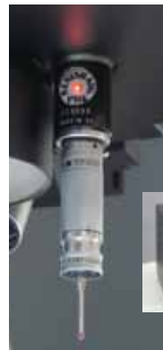
Renishaw® TP200 & PI200 Probe Interface
