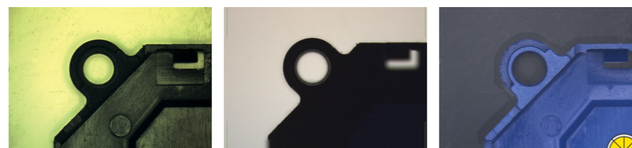
Plastic molded part Under coaxial top light at 0.35x optical magnification
